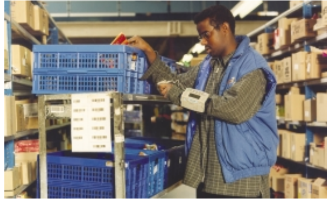
In warehouse and distribution environments, some bar code scanners (like the RS 1 Ring Scanner from Symbol pictured here) are suitable for shipping and receiving, order picking, and inventories/cycle counts. Applications for data capture include tracking work in process and managing cross-dock transfers. (Photo courtesy Symbol Technologies.)
