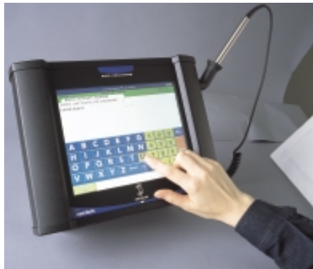
Epic Data's MPT 9100 terminal system implemented at Lockheed Martin features a full-color, 10- x 6-in VGA touchscreen able to present information such as graphical work procedures and CAD drawings to employees on the shop floor. Previous systems offered no inbound information and no access to the corporate intranet.
