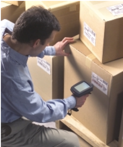
Bar code scanning reduces the workload involved in data-intensive tasks such as tracking inbound inventory and managing material, vehicles, and equipment. Shown is the PDT 7200 portable data terminal from Symbol Technologies, which was designed to withstand the extreme environments found in heavy manufacturing. (Photo courtesy Symbol Technologies.)
